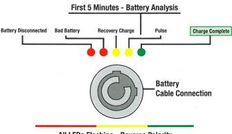
All LEDs Flashing - Reverse Polarity
