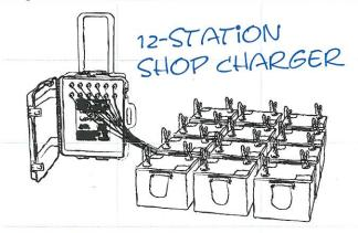
Input Voltage: 110-240 V ac, 15-7.5 A, 50-60 Hz
